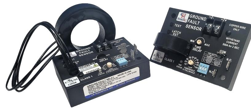
The CR7508 series Ground Fault Sensor, provides a reliable and cost effective method for sensing ground fault currents. Ground fault sensors help to protect equipment and processes from potentially harmful ground fault currents. The CR7508 monitors the differential current of the current carrying wires routed through the current transformer.
