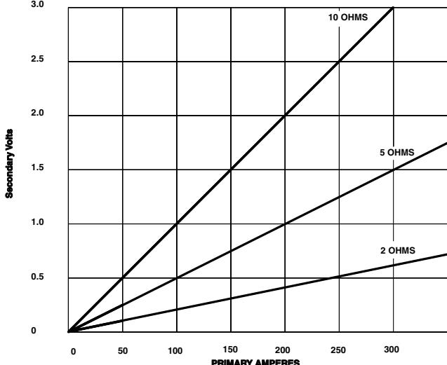
The **610-1000T** Split Core Current Transformer is designed for assembly to an existing electrical installation without the need for dismantling the primary bus or cables. It incorporates a snap fit between the fixed and removable sections.
