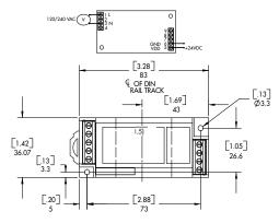
The **CRPS24VDC** Series Power supplies are designed to meter CR Magnetics digital and analog transducers. These switched mode power supplies are compact and efficient with a modern clean looking case.
